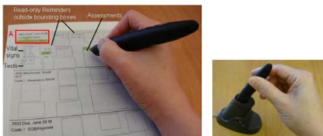
Fig. 7: (left) Personal notes template printed in digital paper with customized layout of bounding boxes and static information, (right) A digital pen docking station.
