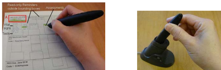
Fig. 4: (Left) Personal notes template printed in digital paper with customized layout of bounding boxes and static information (Right) A digital pen docking station.
